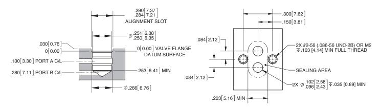
Boss geometries and dimensions shown above are for reference only. All dimensions are in inches [mm].
